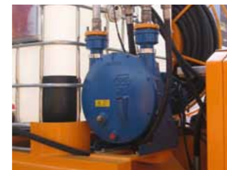
Silicate based hardener – PCM DL18 on shotcrete unit
