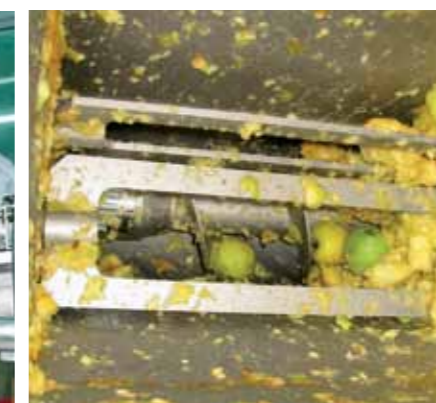
Transfer of whole apples using a screw feed pump for making stewed apple.
