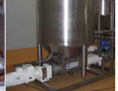
Hopper pump connected to a storage tank
