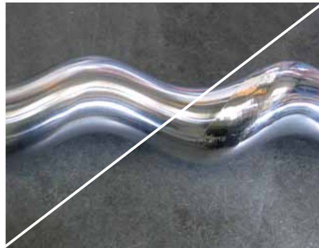
Rotor re-chroming by PCM
