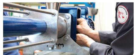
Baseplate: welded steel construction with sloping driptray and drain connection, earthing and lifting attachments.
