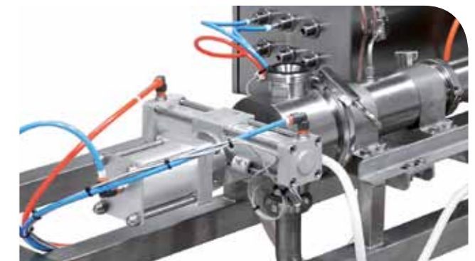
Dosys™ pump driven by Electro-Thrust Cylinder
